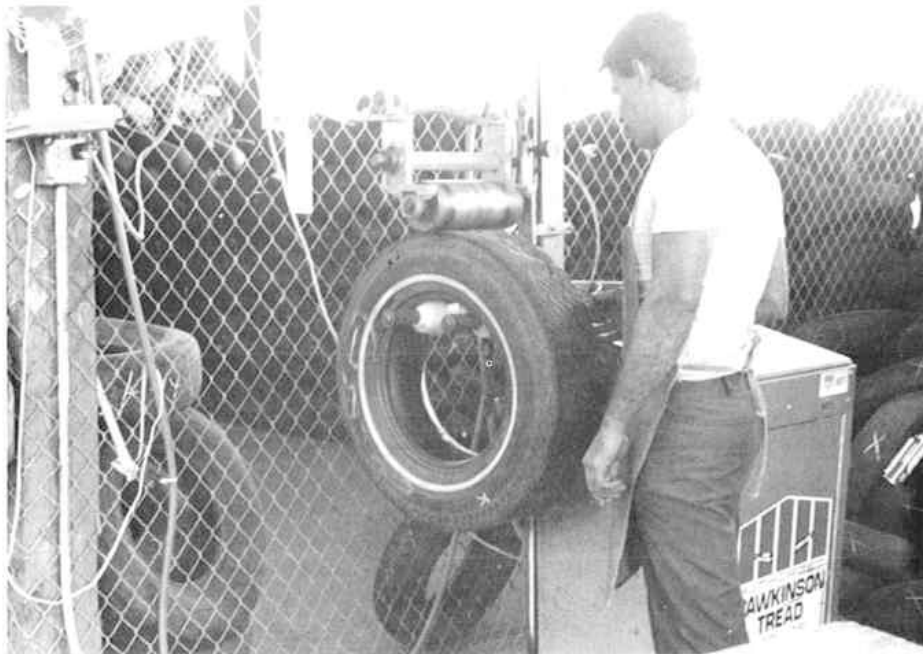
"Outdoor" unit at Tristani, Puerto Rico, inspecting rough graded casings.
