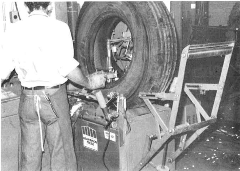
NDT ® at Ray Carr truck tire retreading plant in Harrisonburg, Virginia. Inspects approximately sixty tires per day.
